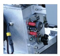
Seven isolated firing circuits are distributed on the F6+ arm and rear, allowing convenient and easy access.
